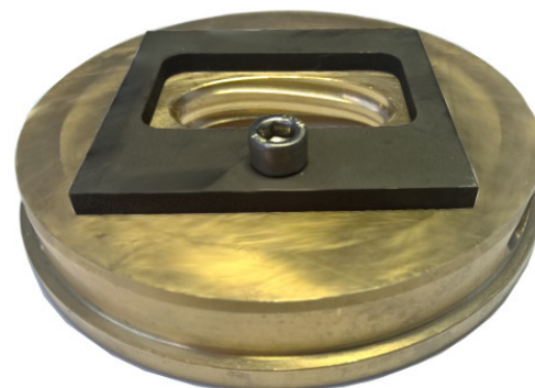
Picture shows flanging die for E65 waveguide
